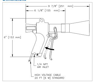
Each Cobra gun is supplied with a standard 20-foot cable for connection to the power supply. A 40-foot cable configuration is also available. Either the G165 or G265 power supply can energize one or two Cobra guns.
